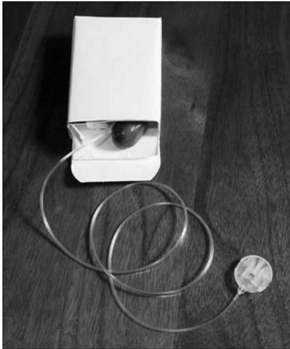
Figure 4-4. A simple prototype of an insulin pump made from a cardboard box and plastic tube, filled with batteries and rocks to approximate weight.
