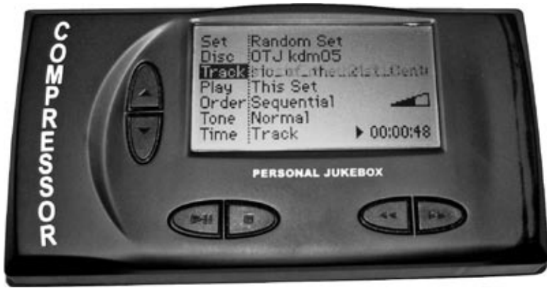
Figure 5-2. The PJB-100 MP3 player offered 5 GB of storage in 1999. Two years later, Apple introduced the iPod, with the same amount of storage.
