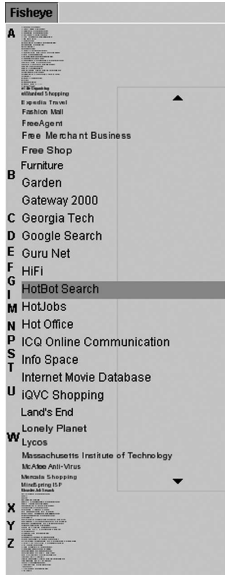
FIGURE 4.20 Focus + context interface schemes distort to show detail in context. (Fisheye Menu courtesy of HCIL at University of Maryland: www.cs.umd.edu/hcil/fisheymenu )
