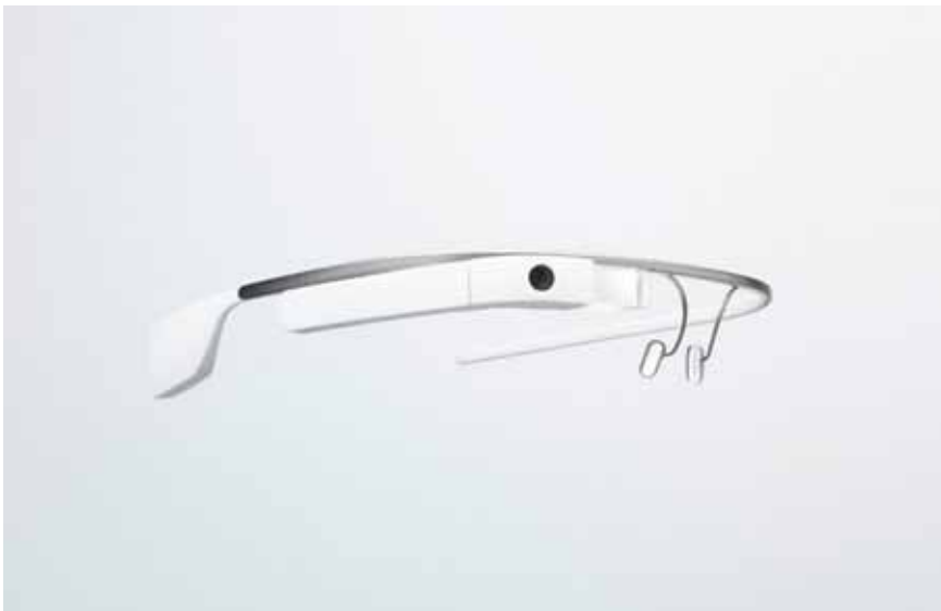
FIGURE 7.1 Google Glass: augmented reality wearable technology ( www.google.com/glass )
