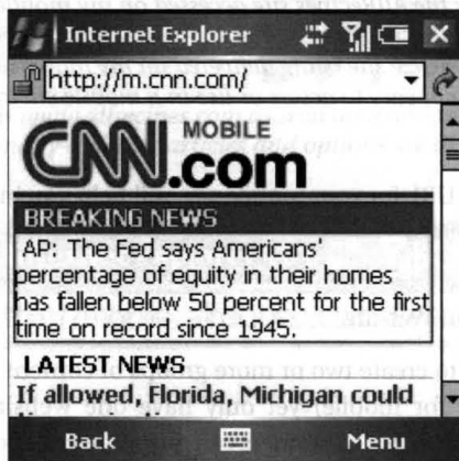
Figure 9.8 This is the CNN Mobile site delivered on my mobile. I entered the same URL as I did from my desktop computer, and the CNN site understood that I was looking at it from a mobile browser, hence sending the mobile version.
