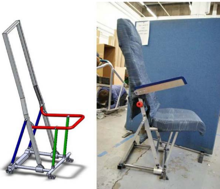
Figure 10.2 CAD model and functional prototype of an innovative economy-class airline seat
