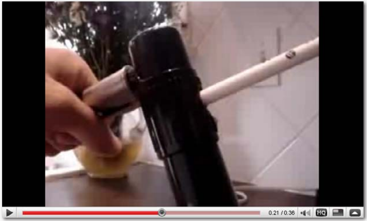
Figure 1-2. Viral videos demonstrated how to pick Kryptonite bike locks with only a Bic pen.
